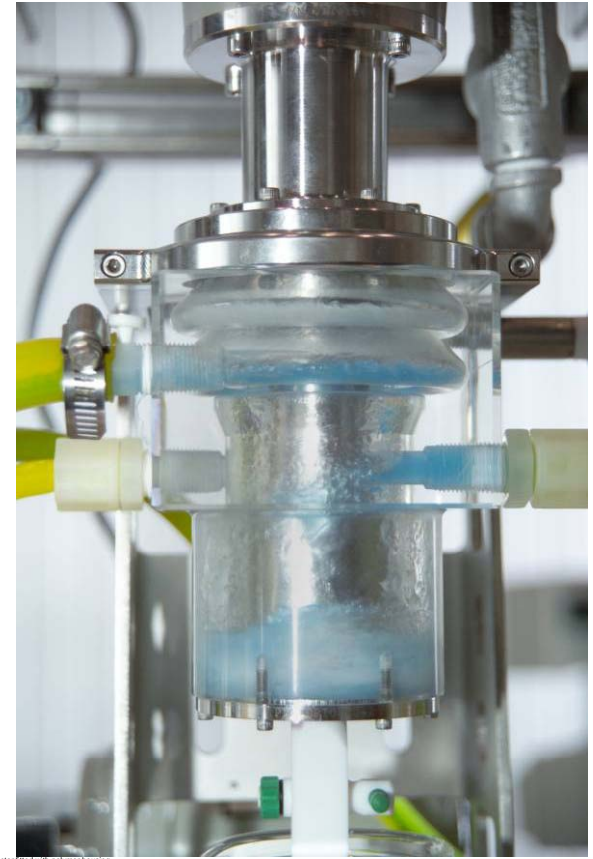
Contactor fitted with polymer housing
